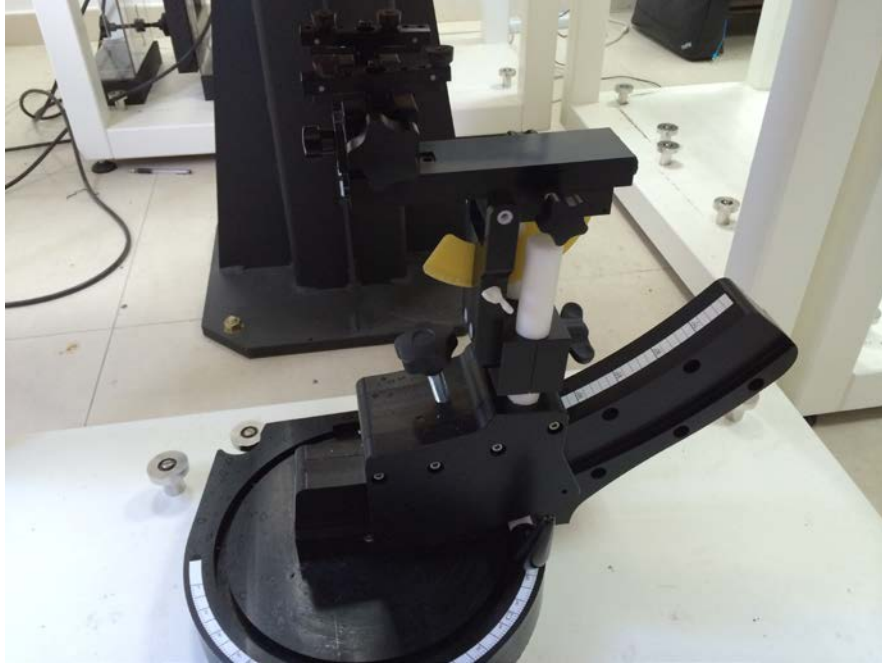
Device holder supplied by SPEAG
