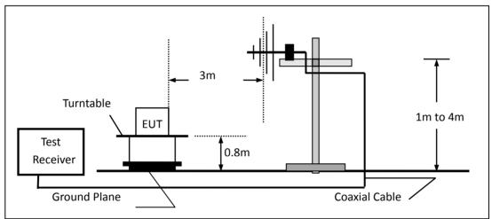
(c) For radiated emissions above 1000MHz
