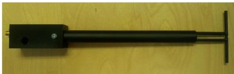
Figure 1 – MVG COMOSAR Validation Dipole
