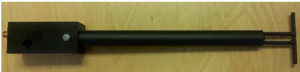
Figure 1 – MVG COMOSAR Validation Dipole
