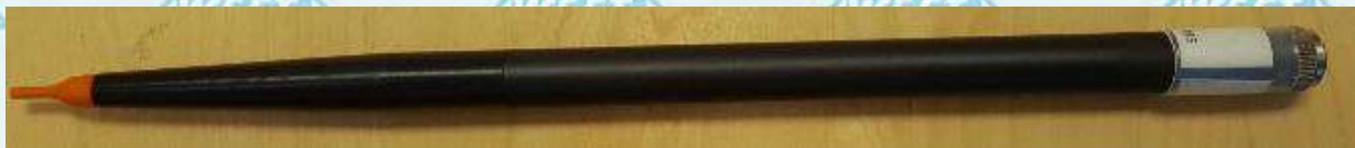
Figure 2 – MVG COMOSAR Dosimetric E field Dipole
