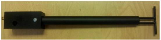
Figure 1 - MVG COMOSAR Validation Dipole
