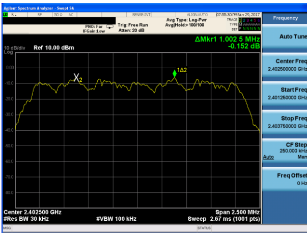
(3Mbps) Channel Separation plot on channel 39-40
