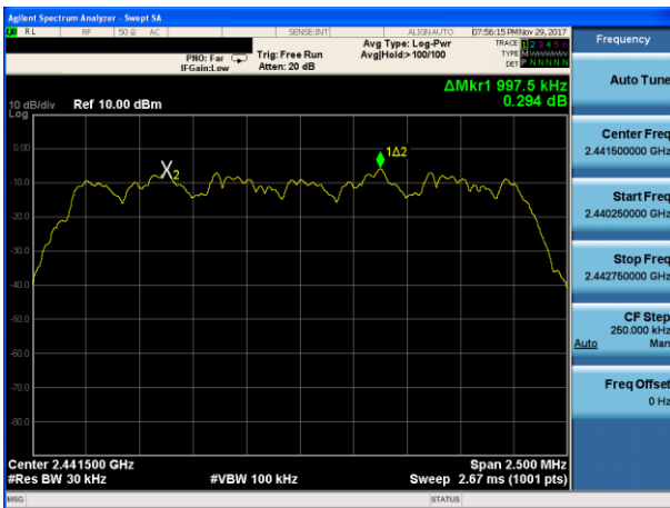
(3Mbps) Channel Separation plot on channel 77-78
