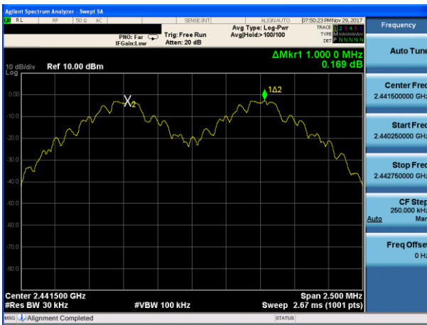
(1Mbps) Channel Separation plot on channel 77-78
