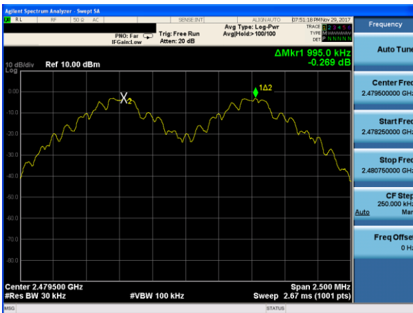
(1Mbps) Channel Separation plot on channel 77-78
