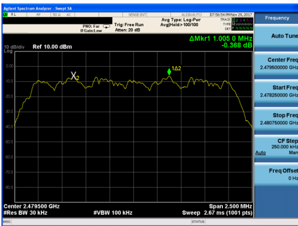
(3Mbps) Channel Separation plot on channel 77-78
