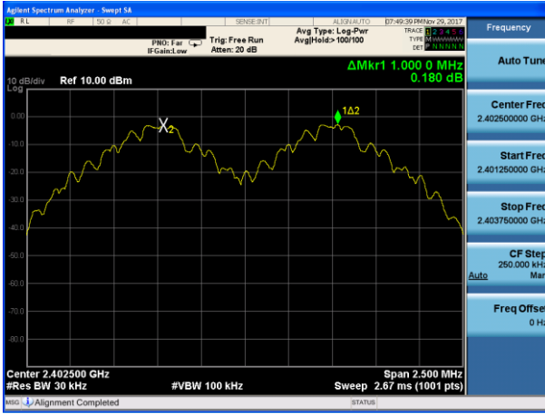
(1Mbps) Channel Separation plot on channel 39-40
