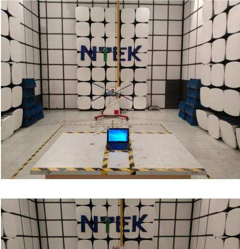
Radiated Measurement Photos ( original battery )
