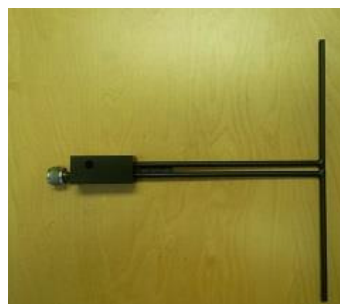
Figure 1 – MVG COMOSAR Validation Dipole
