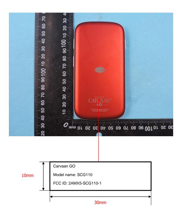
Note: This label is silk creen on the surface of the prototype
