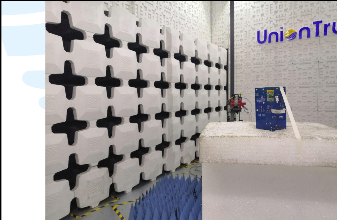
Radiated emission Test Setup (Above 1 GHz)
