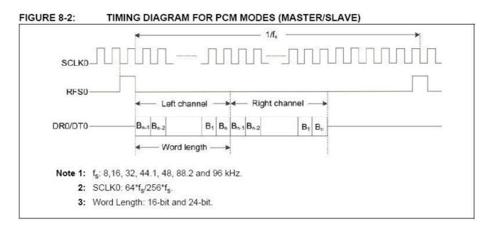
Figure 8-3 illustrates the timing diagram of the audio interface.
