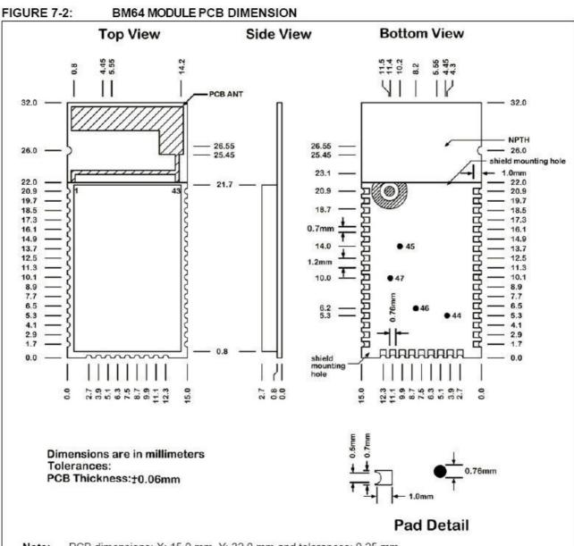
Note: PCB dimensions: X: 15.0 mm, Y: 32.0 mm and tolerances: 0.25 mm.
