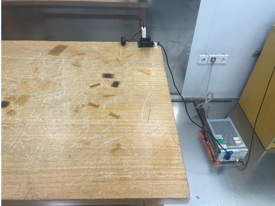
Photo of Setup for Radiated Emission (30MHz~1GHz)
