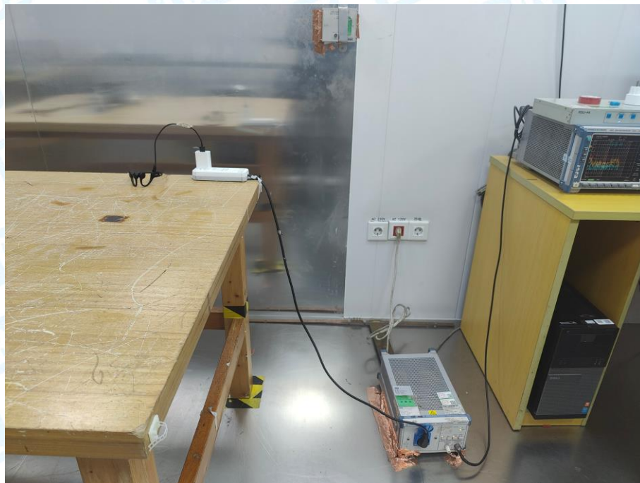
Photo of Setup for Conducted Emission
