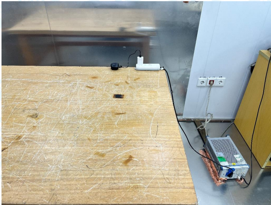
Photo of Setup for Conducted Emission
