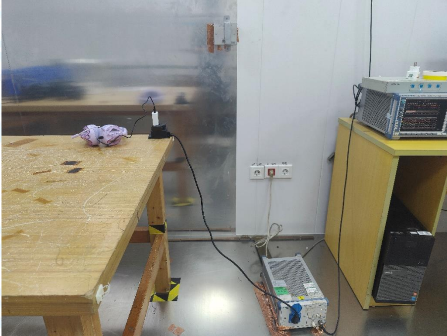
Photo of Setup for Radiated Emission (30MHz~1GHz)
