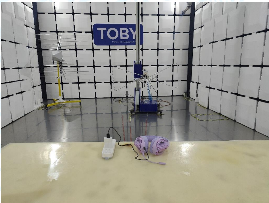
Photo of Setup for Radiated Emission (30MHz~1GHz)
