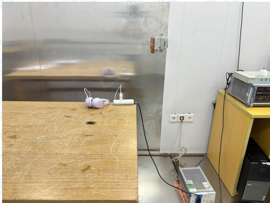
Photo of Setup for Conducted Emission
