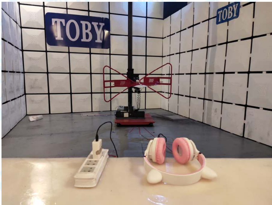
Photo of Setup for Conducted Emission
