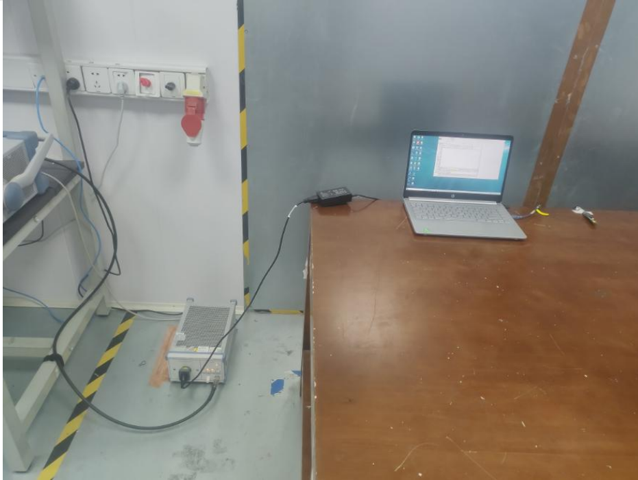
Conducted emissions at AC power line (150kHz-30MHz)
