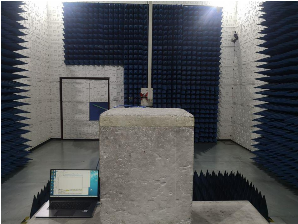
RADIATED EMISSION TEST SETUP ABOVE 1GHZ
