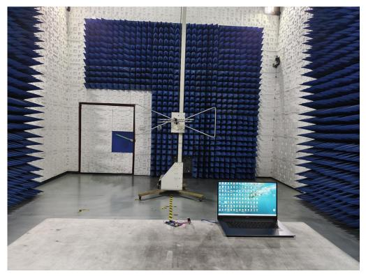
RADIATED EMISSION TEST SETUP ABOVE 1GHZ
