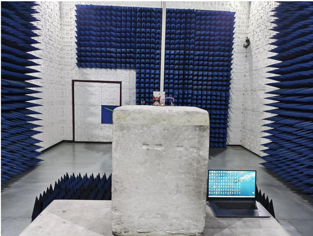
RADIATED EMISSION TEST SETUP ABOVE 1GHZ
