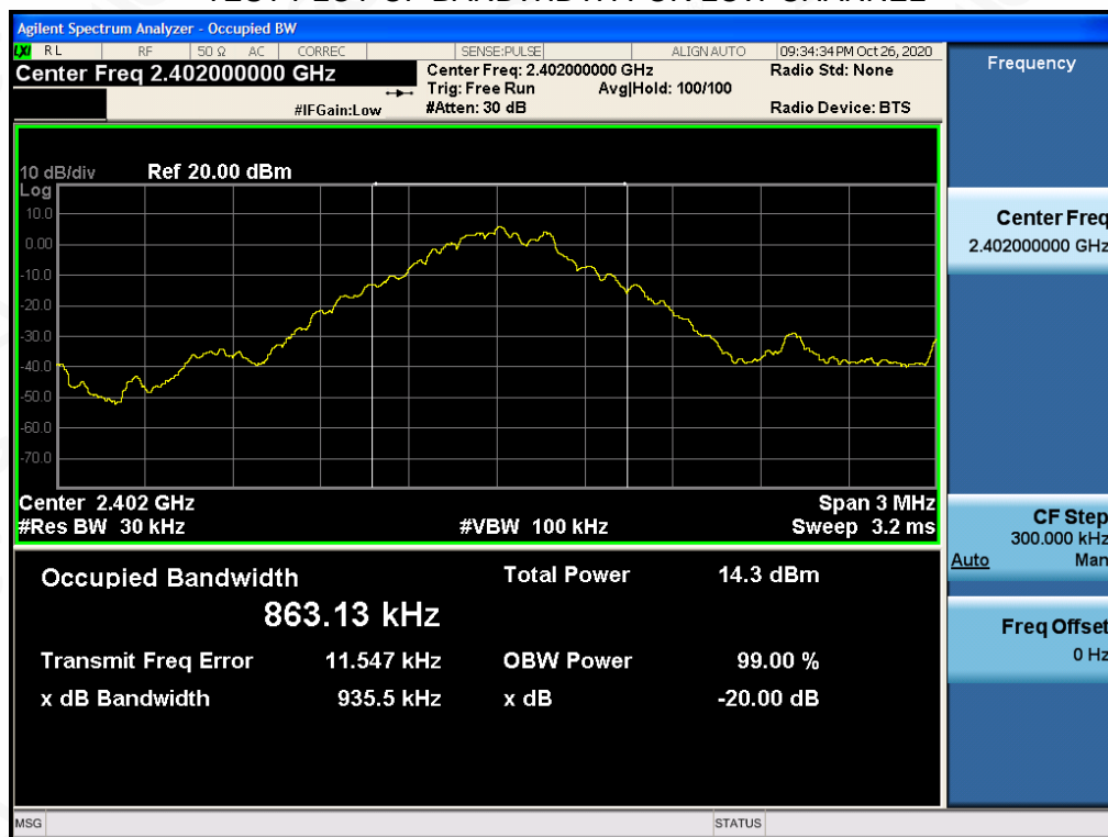
TEST PLOT OF BANDWIDTH FOR LOW CHANNEL
