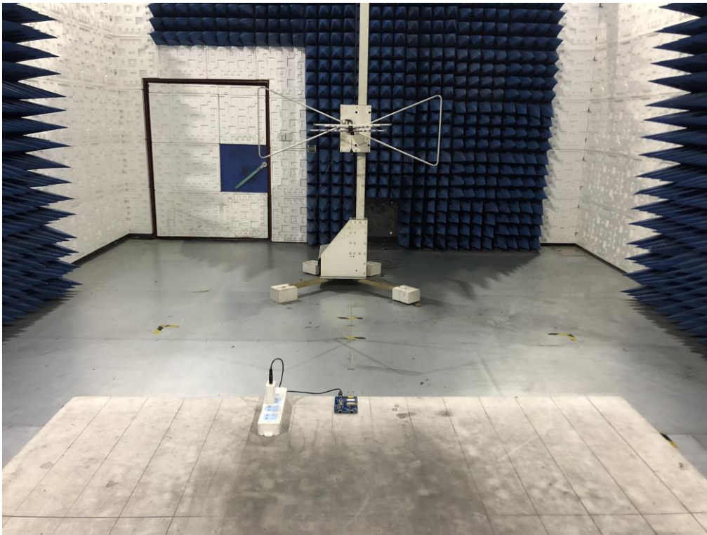
RADIATED EMISSION TEST SETUP ABOVE 1GHZ
