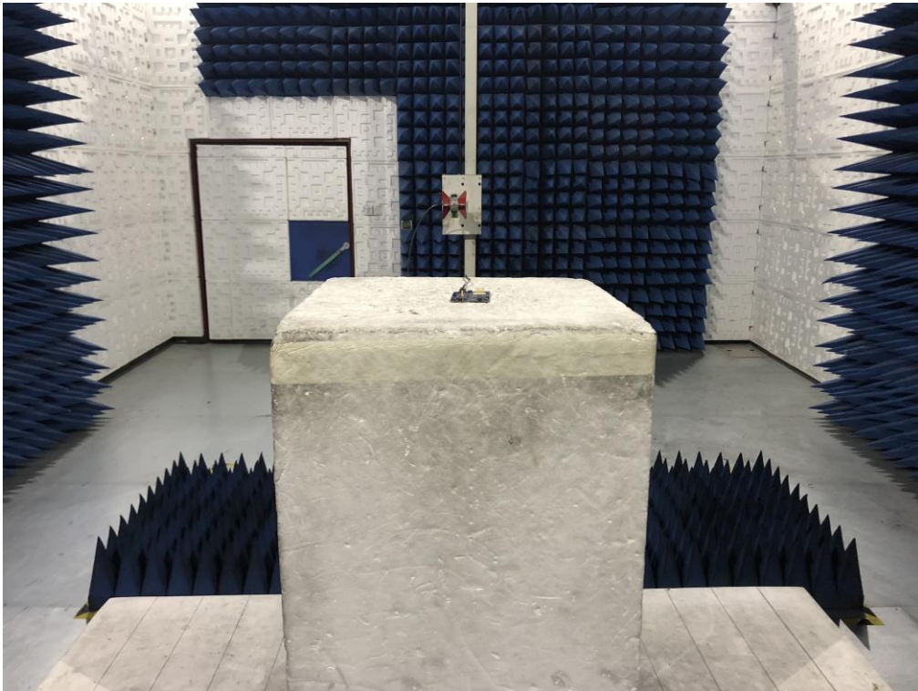
RADIATED EMISSION TEST SETUP ABOVE 1GHZ
