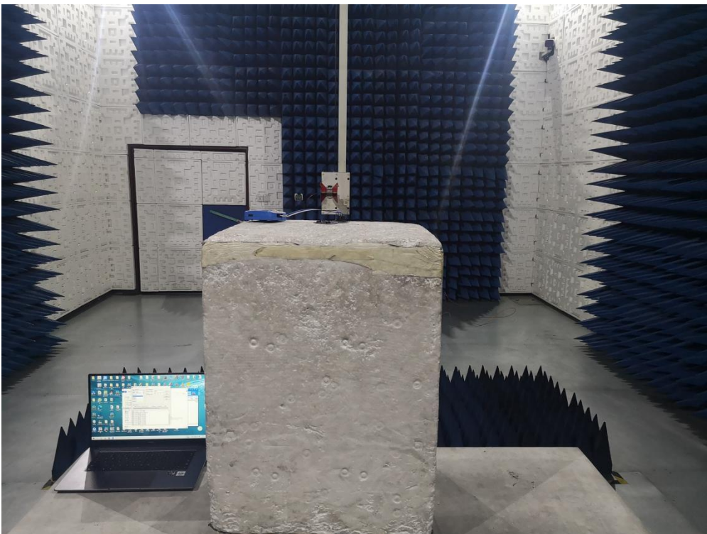
RADIATED EMISSION TEST SETUP ABOVE 1GHZ
