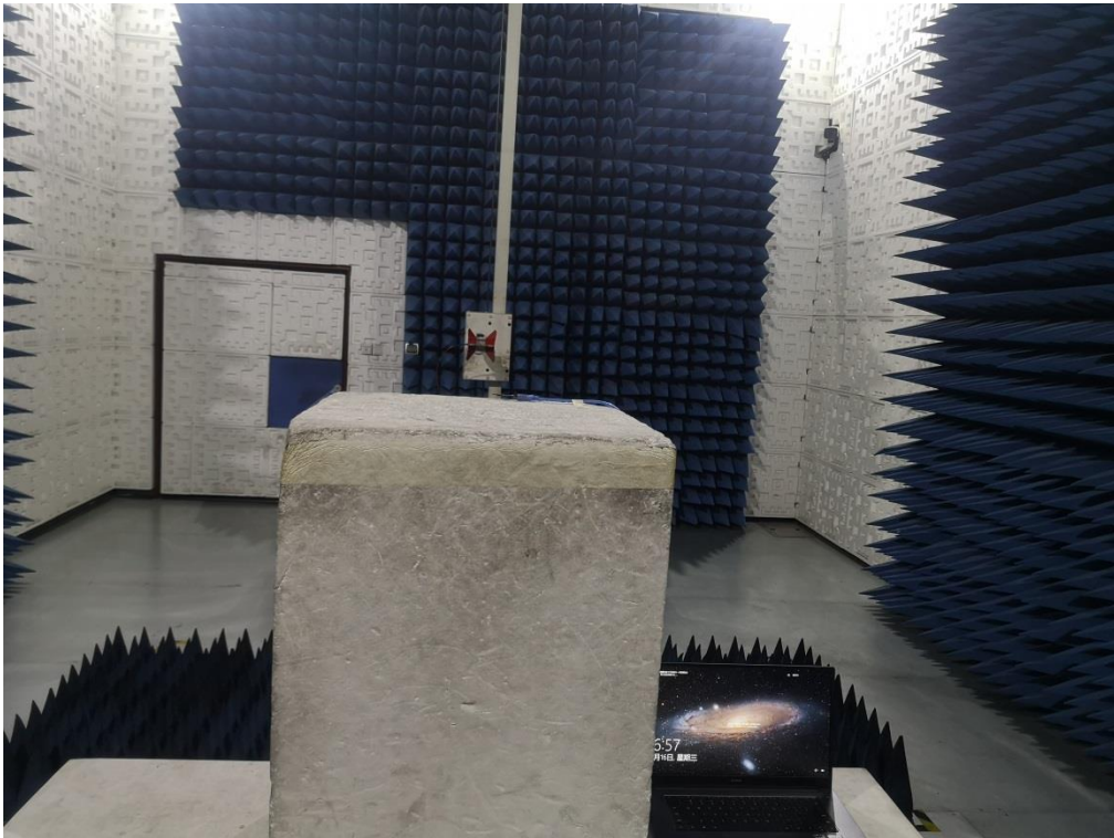
RADIATED EMISSION TEST SETUP ABOVE 1GHZ
