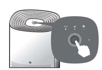
Press the Mode button to enter the turbo mode, to increase the fan speed when air pollution is heavy
