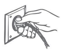
Plug in the power cord to the wall socket, make sure all three pins are connected , so that the system is properly earthed/ granded (AC110V – 240V 60/50Hz)
