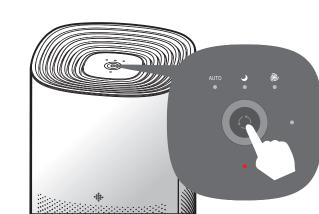
Press and hold Power On/Off button for 3 seconds to turn off the machine and the red LED is come on
