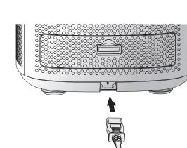
Plug in the power cord into the back of the machine
