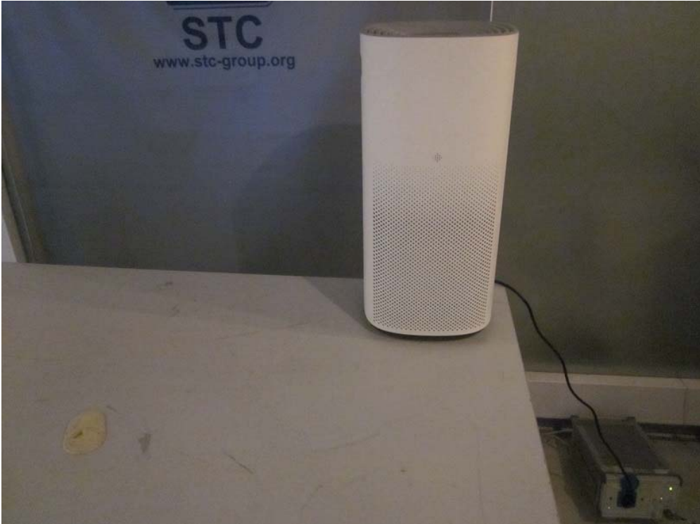
Measurement of Conducted Emission Test Set Up
