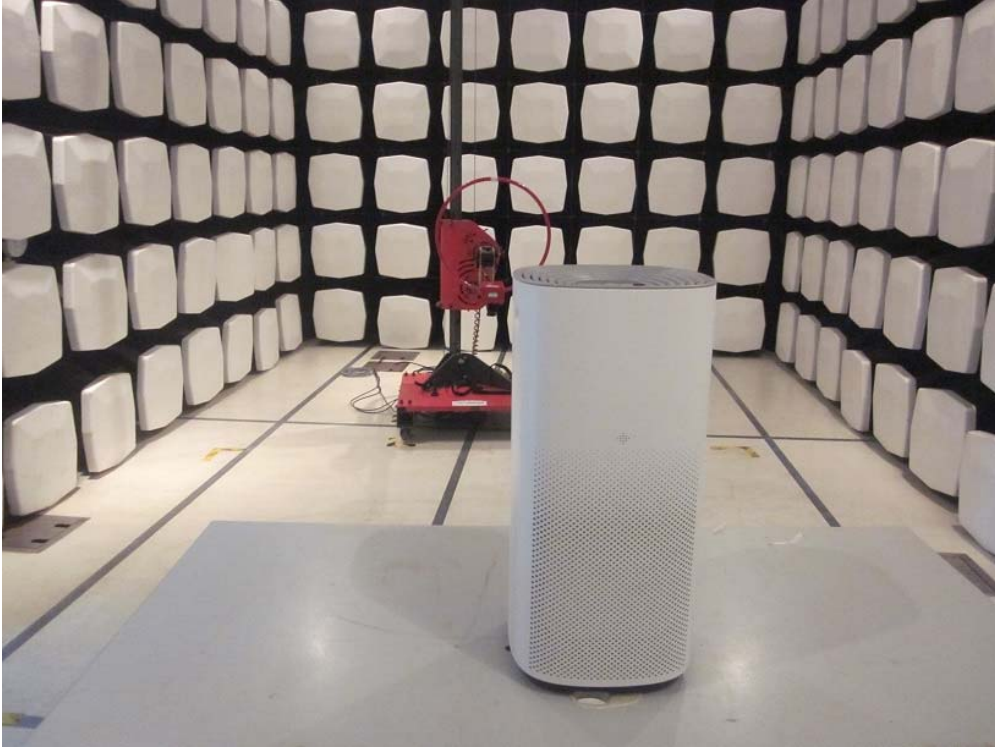
Measurement of Radiated Emission Test Set Up
