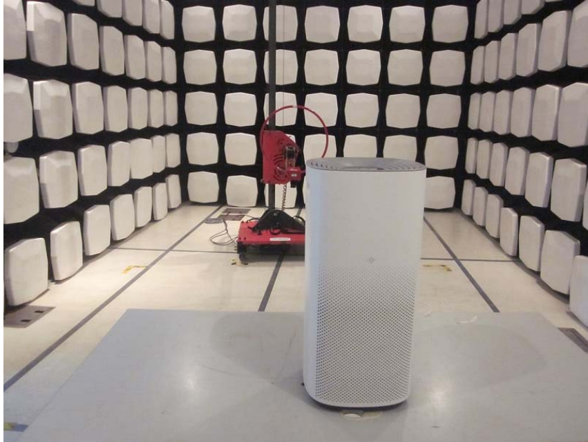
Measurement of Radiated Emission Test Set Up
