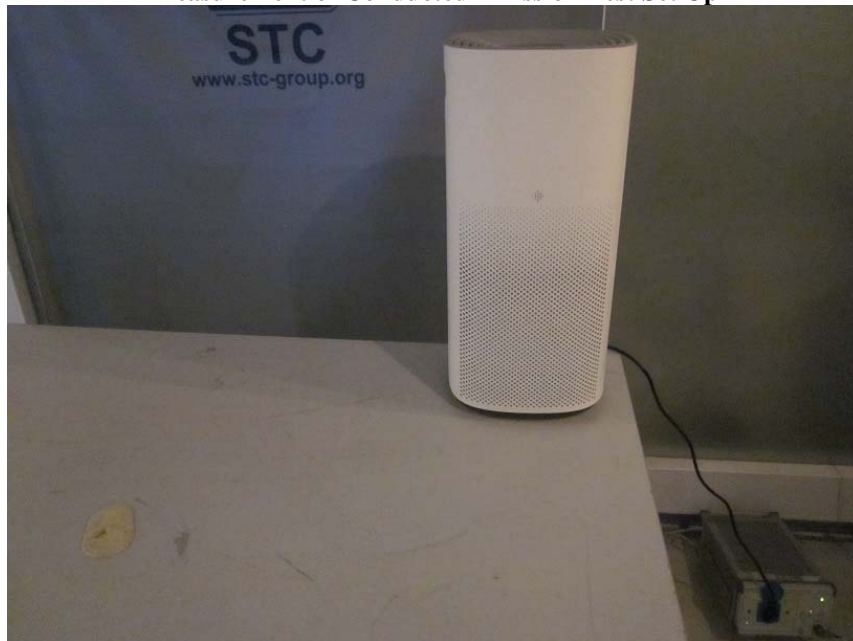
Measurement of Conducted Emission Test Set Up
