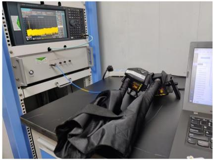
RF Radiated Test(30-1000MHz)
