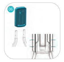
Place the back-support plate on top of the rods. Fix it with the screws and gaskets (Items No. 12 and 13). Temporarily do not tighten them completely - only turn each of them 3 times.
