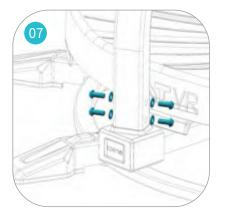
Install the screws and gaskets at the bottom of the rods (Items No.14 and 15). Note:Tighten them well to avoid safety hazards.
