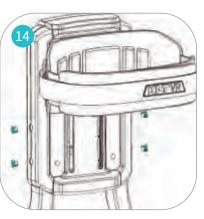
If the beam continues to return to the same position, lower the opposite side of the platform by adjusting the corresponding screw (turn it right). Once leveled, tighten the upper nuts.
