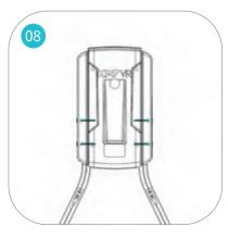
Now, tighten the back-support screws. Note: Tighten them well to avoid safety hazards.
