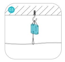
Hang the wire pulley onto the hook.
