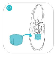
The slot at the back of the sensor fits into the socket sewed into the shoe.
