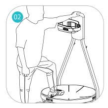
When entering the platform, grab the upper edge of the back-support plate for better stability. Mind that the structure is rotational and may move.
