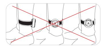
II. Warning: The picture above shows improper placement of the sensors. Puting the sensors on upside down will disable their normal operation.
