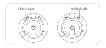
03. **Waist sensor mag calibration:** When used for the first time, the waist sensor requires to collect the location data to complete the calibration process. Select 'Waist Mag Calibration' in KAT Gateway and follow the instructions on the screen. In order to start the calibration process, select 'Waist Mag Calibration' in KAT Gateway and follow the instructions on the screen.
