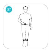
07. **Waist sensor calibration:** After starting a game (Please, confirm that SteamVR started as normal), put on your headset, keep your feet together and look straight to ensure the direction of your face is the same as the direction of your body. Then, press the 'Calibration Button' right at the center of the waist sensor (Or directly in the dashboard of KAT Gateway) to complete the calibration process.
