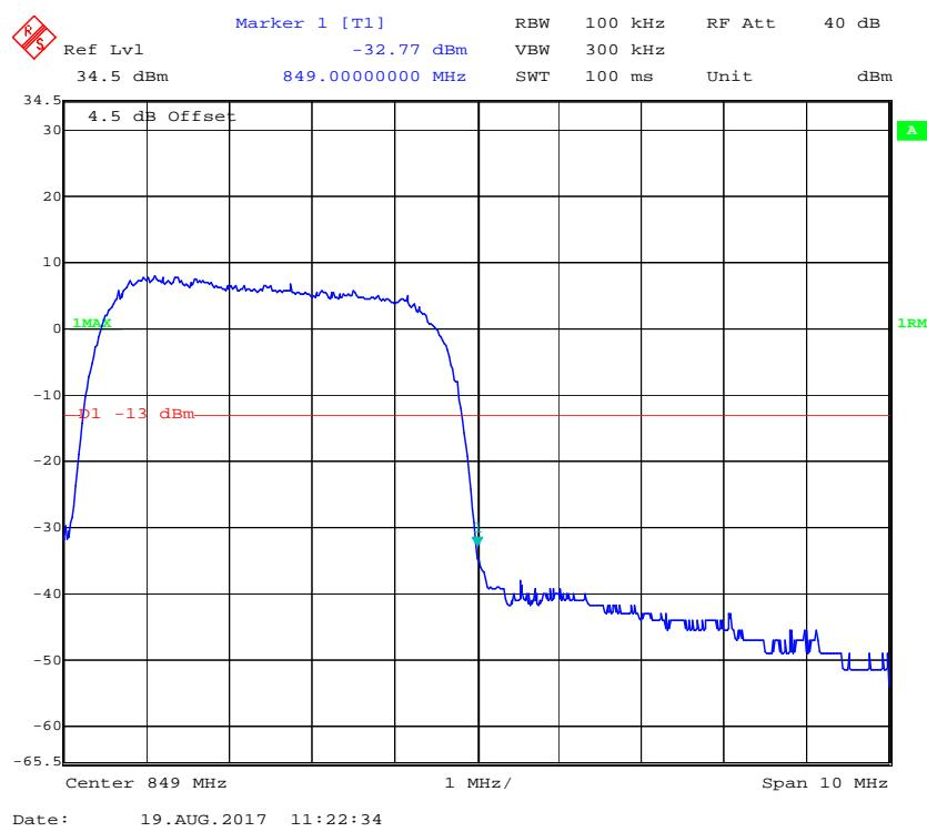
**PCS Band, Left Band Edge for GSM (GMSK) Mode**
