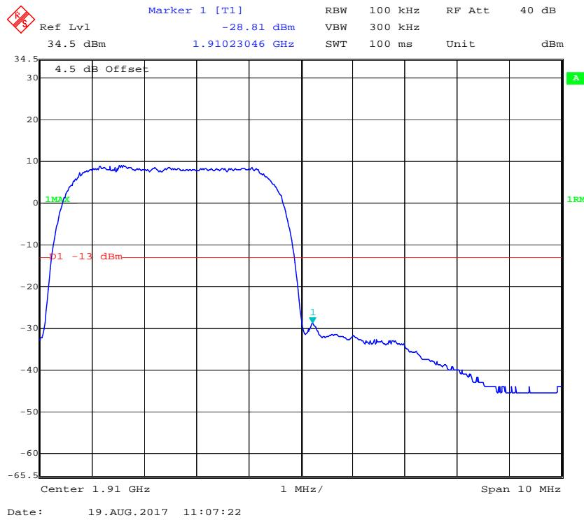
**PCS Band, Left Band Edge for HSDPA (16QAM) Mode**
