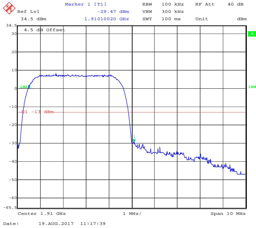
**PCS Band, Left Band Edge for HSUPA (BPSK) Mode**
