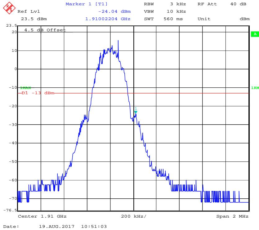
**PCS Band, Left Band Edge for RMC (BPSK) Mode**
