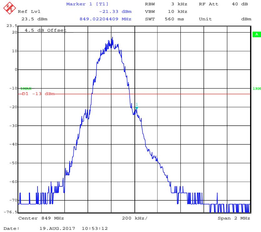
**Cellular Band, Left Band Edge for RMC (BPSK) Mode**
