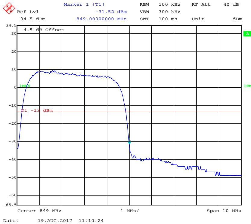
**Cellular Band, Left Band Edge for HSDPA (16QAM) Mode**
