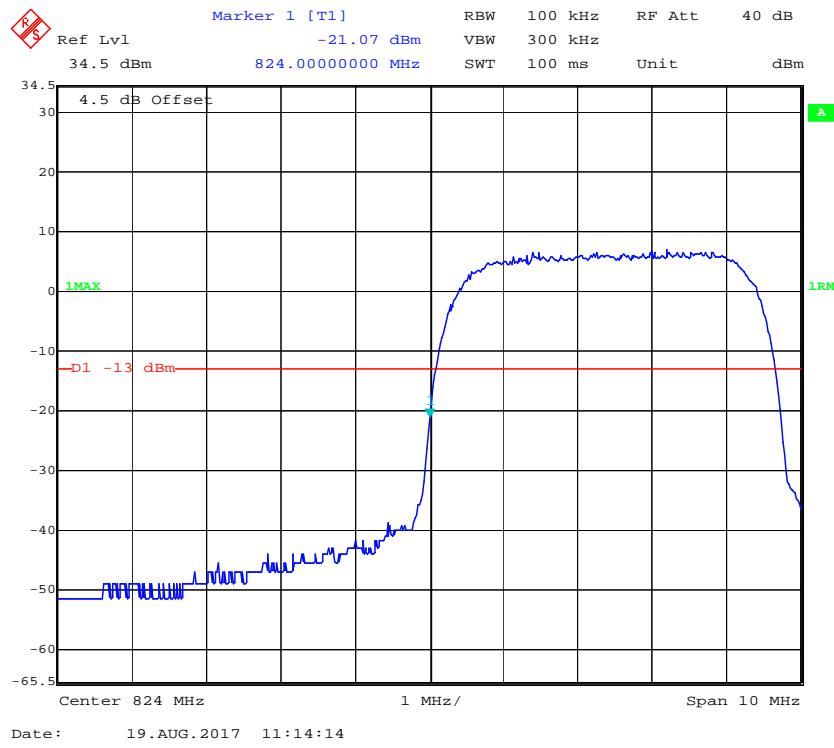
**Cellular Band, Right Band Edge for HSDPA (16QAM) Mode**
