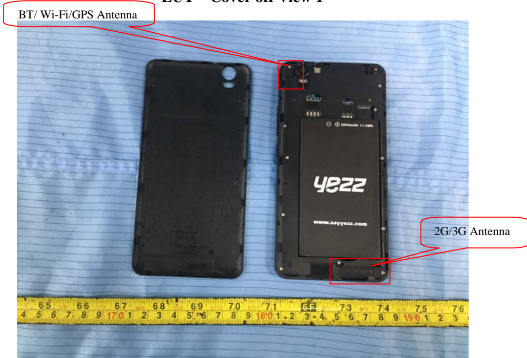
EUT – Cover off View 1
