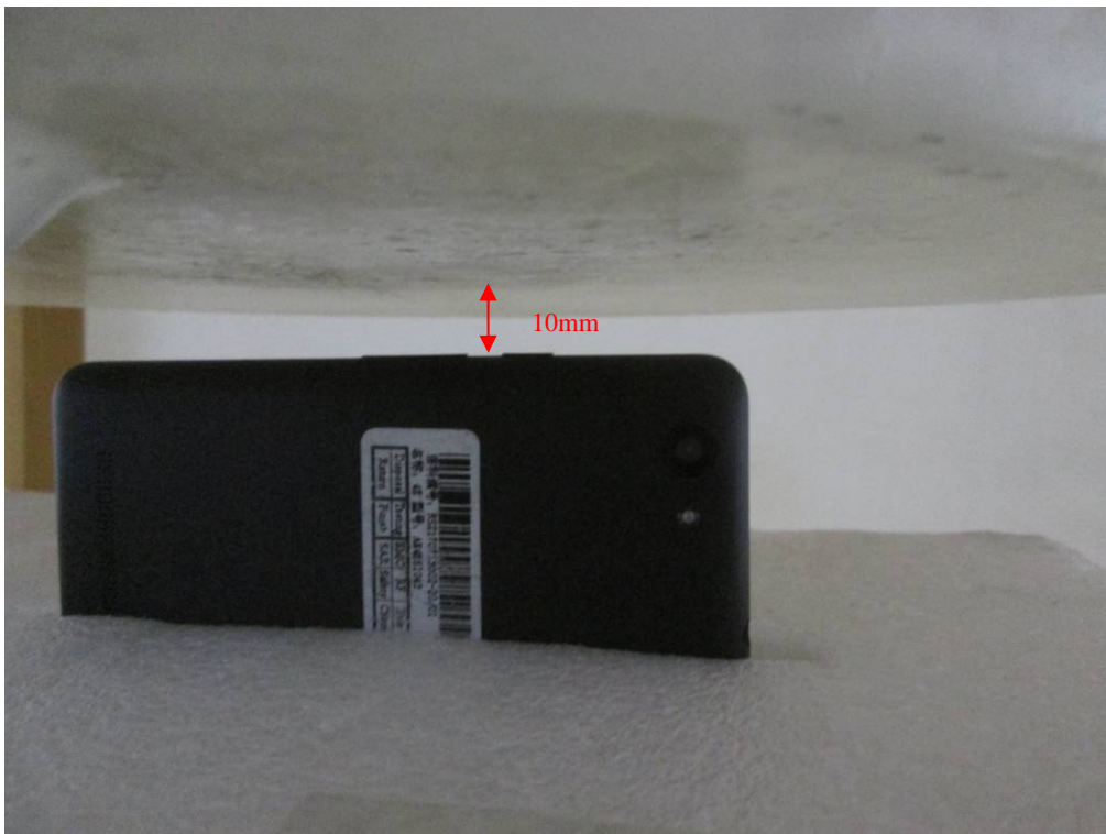
Body-worn Right Setup Photo (10mm)
