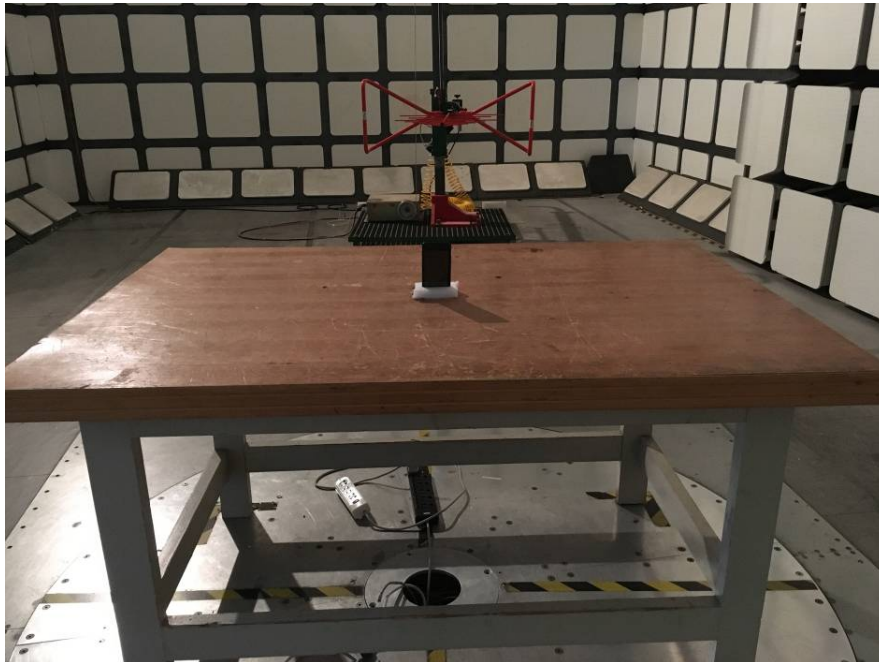
Radiated Emissions View (Below 1 GHz)
