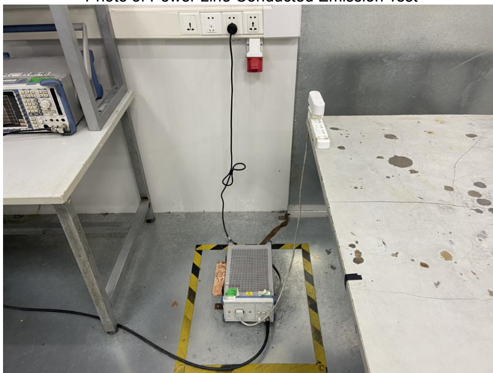
FCC ID: 2AMV5SK522-W Photo of Power Line Conducted Emission Test
