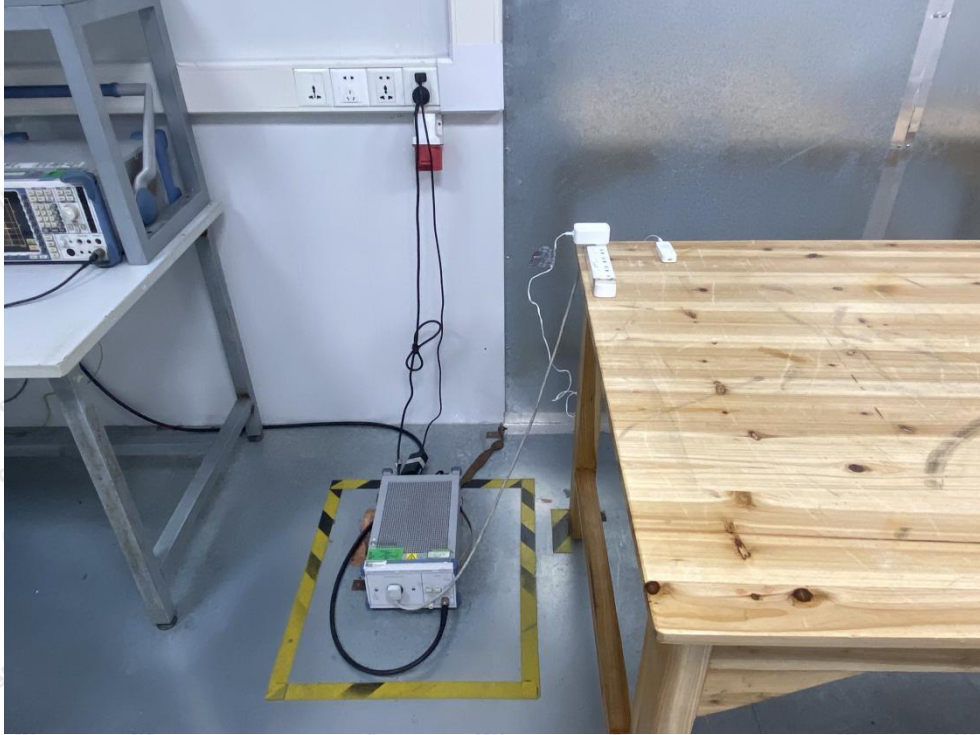
Photo of Conducted Emission Measurement
