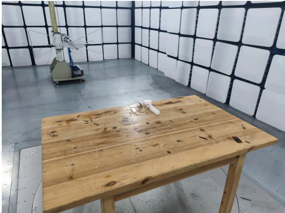
Photo of Radiation Emission Test
