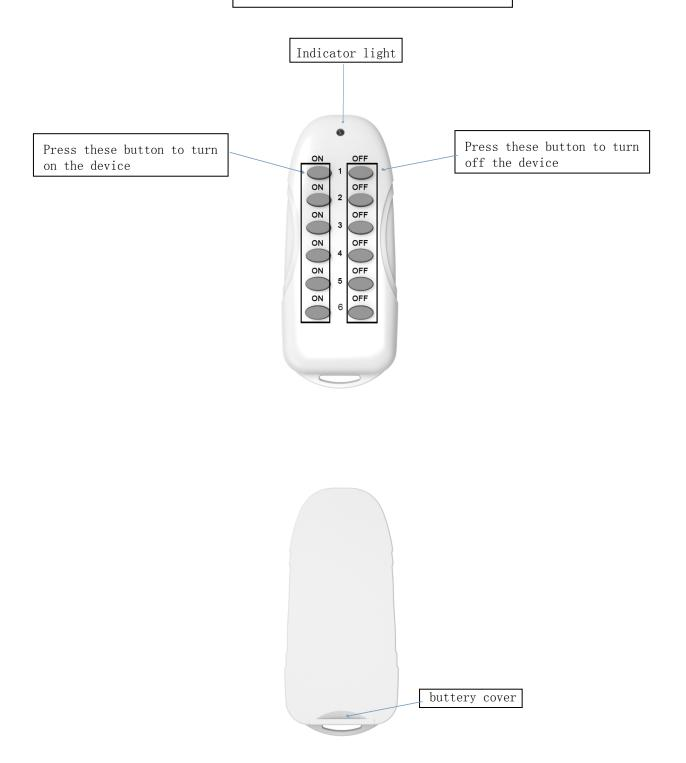
This is a transmitter used for control the device, the device maybe a light, fixed camera, home appliances and so on. The receiver usually connected the control switch which can control the device on and off.
