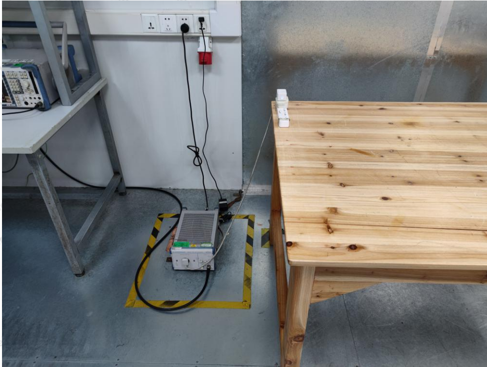
Photo of Power Line Conducted Emission Test
