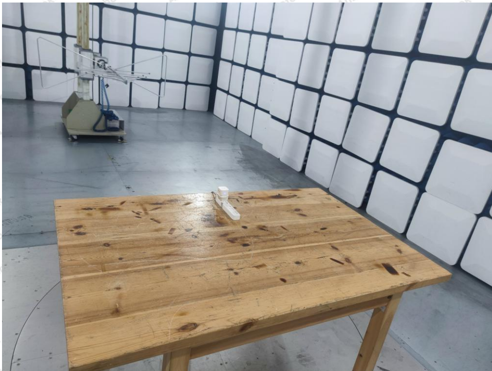
Photo of Radiation Emission Test
