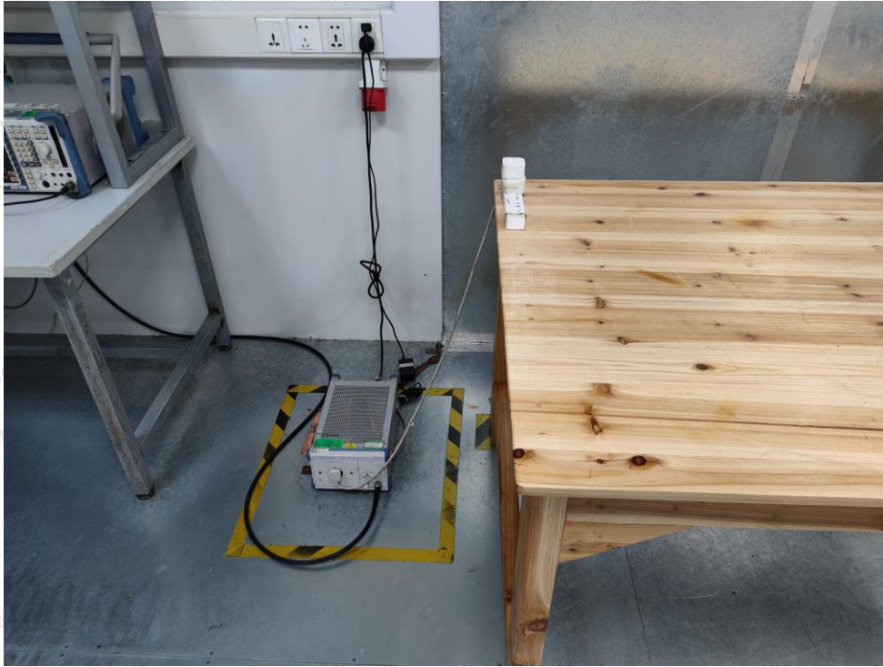
Photo of Power Line Conducted Emission Test
