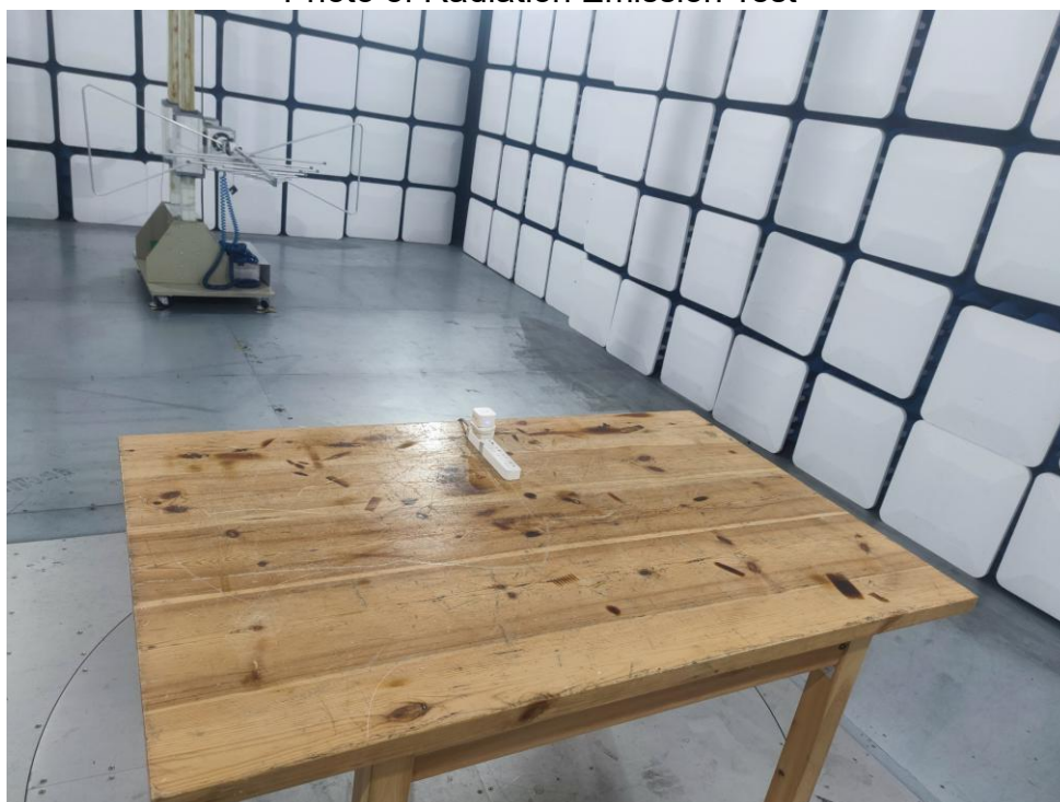
Photo of Radiation Emission Test
