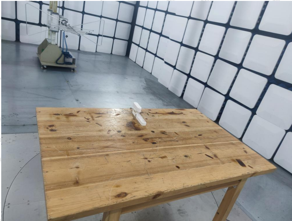
Photo of Radiation Emission Test
