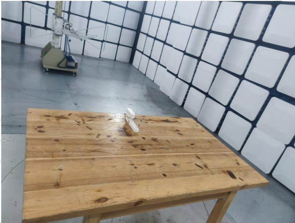
Photo of Radiation Emission Test
