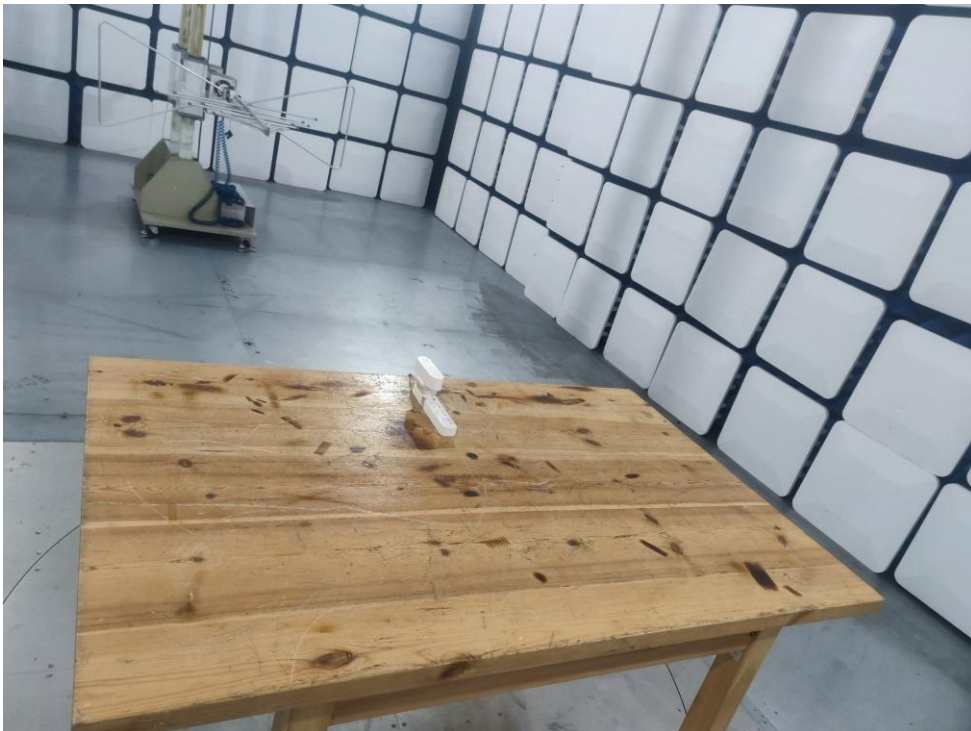
Photo of Radiation Emission Test
