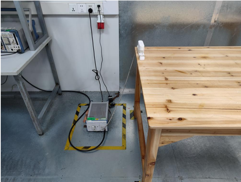
Photo of Power Line Conducted Emission Test
