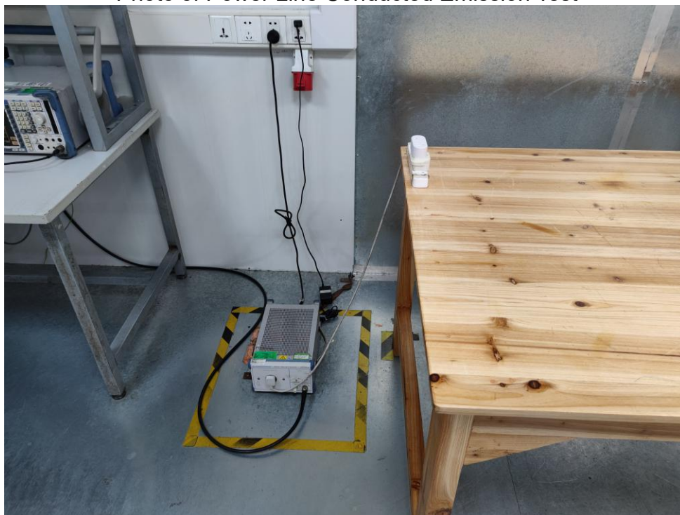
FCC ID: 2AMV5-SK513-W-A Photo of Power Line Conducted Emission Test
