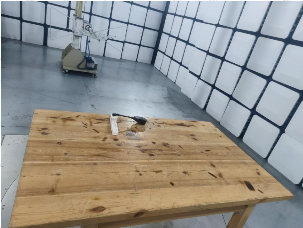
Photo of Radiation Emission Test
