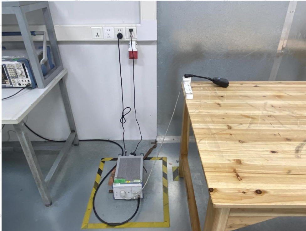
Photo of Power Line Conducted Emission Test
