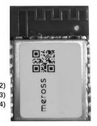
PIN16--UTX0 PIN15--URX0 PIN14--GPIO20(PWM0) PIN13--GPIO19(PWM7) PIN12--GPIO18 PIN11--GPIO12/NC PIN10--GPIO0 PIN9--GND
