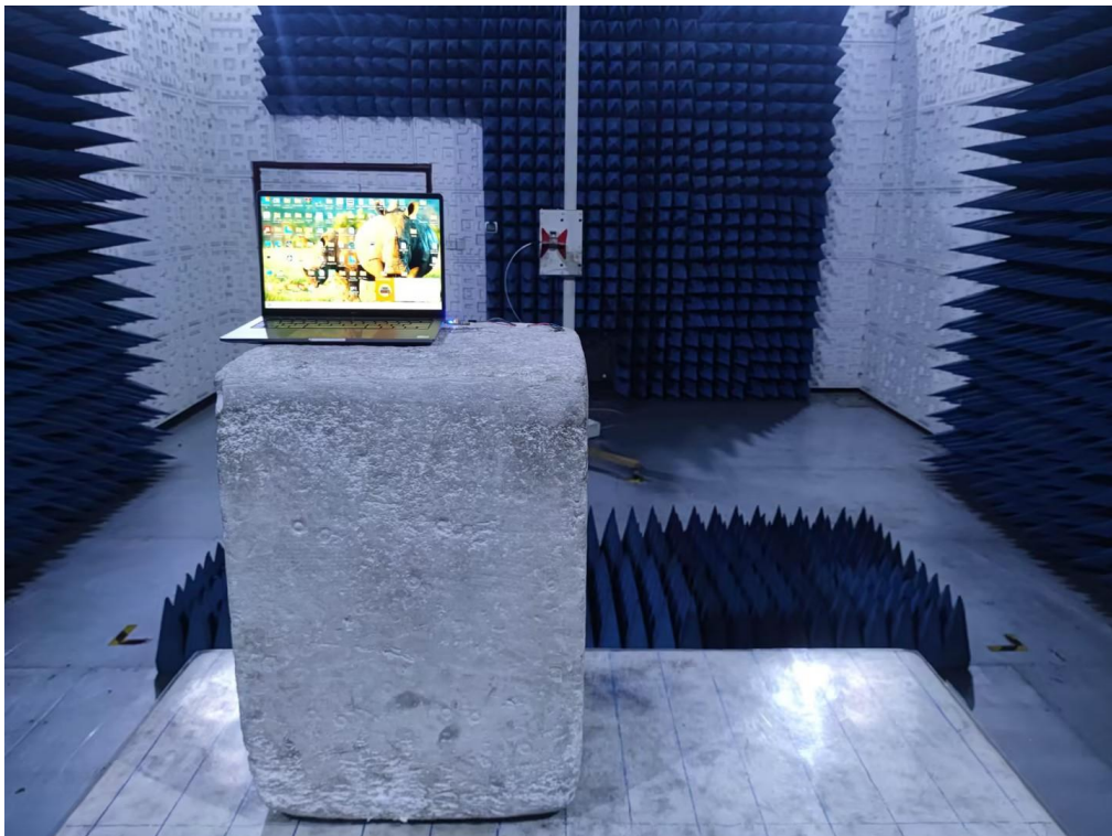
RADIATED EMISSION TEST SETUP ABOVE 1GHz
