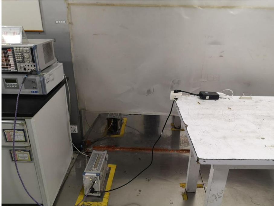
Conducted Emissions Test Setup
