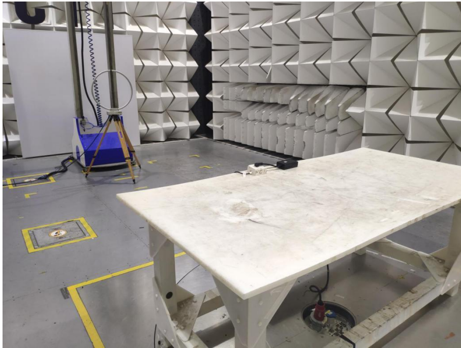
Radiated spurious emission Test Setup-1(Below 30MHz)
