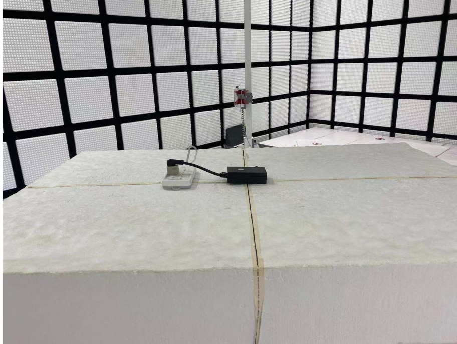
Radiated spurious emission Test Setup-3(Above 1GHz)
